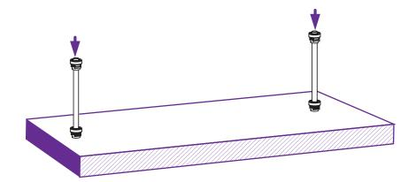
• Adjust the bottom and top donuts to compensate for a crooked pipe anchor.
